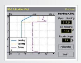
Rudder activity and heading changes are displayed. Autopilot settings can directly be changed.
