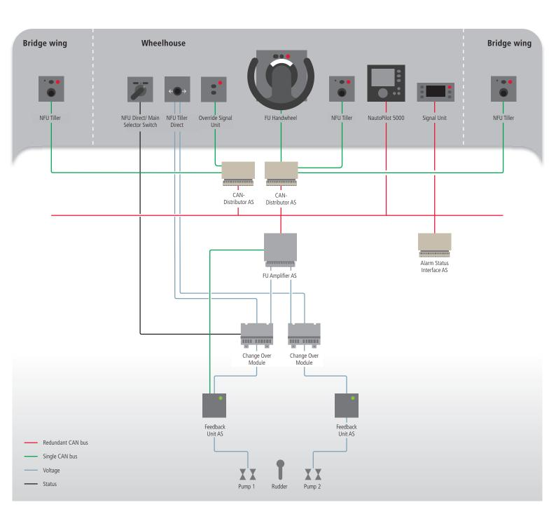
In "NFU Direct" mode the NFU Tiller direct operates the valves/ pumps of the steering gear directly. The override signal unit is used for override of autopilot or other controls. In "Main" mode the FU Handwheel and therefore the CAN bus based steering gear control system is activated. Other controls can simply be activated at the steering control position with a take-over function. The valves/pumps are operated with one FU Amplifier.
