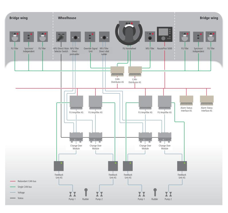
In "NFU Direct" mode two NFU Tiller direct operate the valves/ pumps of the steering gear directly. Both rudders are controlled independently from each other. The override signal unit is used for override of autopilot or other controls.
