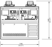
GMDSS A3 Radio Station Small Deckstand
