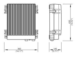
150 W MF/HF Transceiver Weight 19 kg
