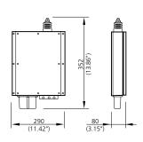
Antenna Tuning Unit (ATU) Weight 3.3 kg
