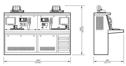
GMDSS A3 Radio Station Large Deckstand
